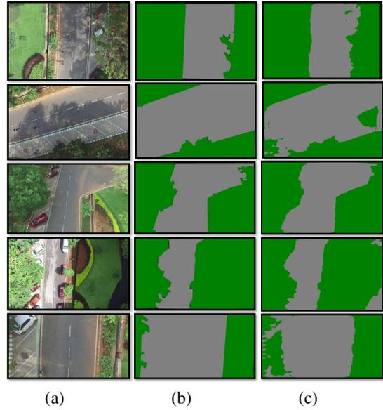
Fig. 7. Semantic segmentation results of U-Net. (a) Original images (b) Ground truth images (c) U-Net segmentation results
