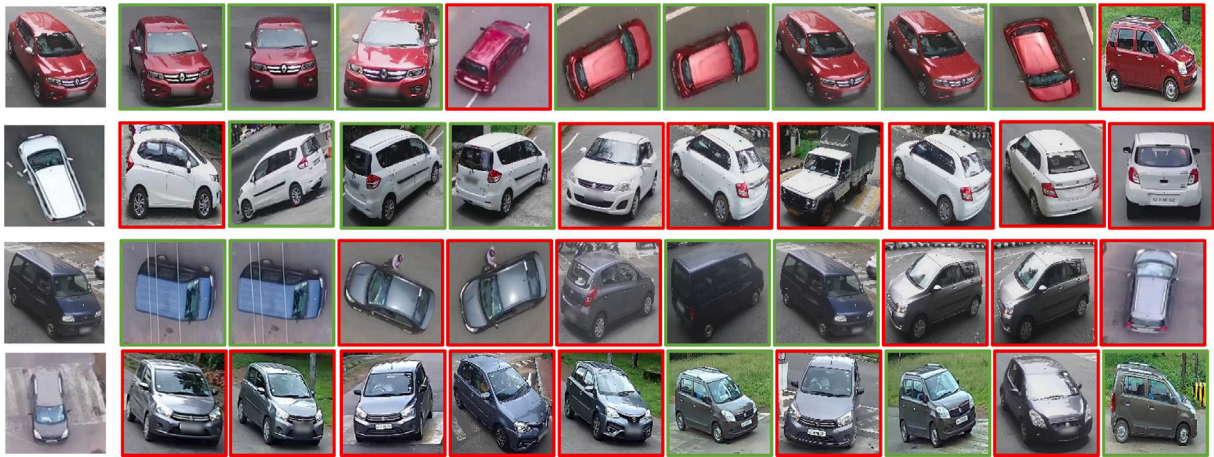
Fig. 10. The retrieval of the top 10 identical vehicles for a given query. At each row, the first image is the query for which the top-10 identical vehicles observed across CCTVs and UAV are retrieved. A retrieved identical vehicle with a green border is a positive match, and a vehicle with a red border indicates a vehicle that has been incorrectly re-identified.
